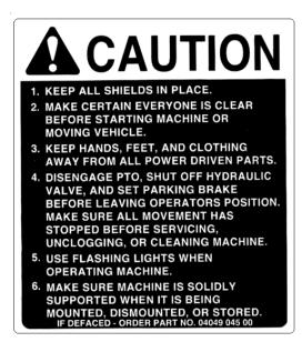
This decal appears on the left end, or the right end of the spreader trough. It cautions all to observe general safety procedures when operating this equipment.
