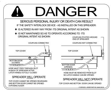
This decal appears on the back of the spreader cover plate at the right end of the spreader. It alerts all to the danger associated with the improper use of the Safety Interlock Device.
