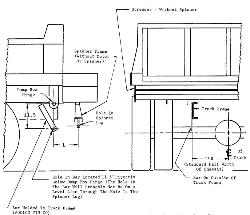
Note - If Hole Under Spinner Frame Cannot Be Located As Shown, Modifications Must Be Made To Spinner Frame - See Instructions!
