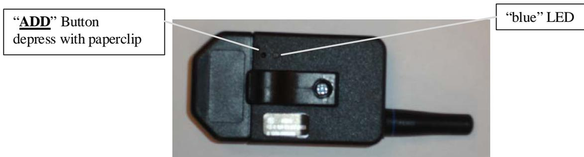
**Fig. 2: Transmitter Back Button Assignments**
