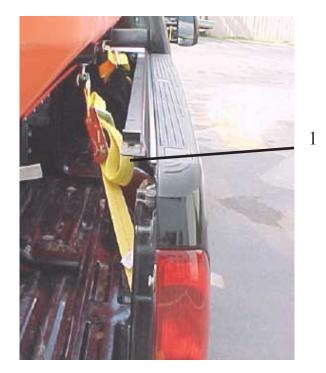
\* Photo for hold down reference only, not MDV installation. MDV cannot be installed in pick-up type vehicles.
