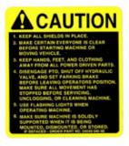
This decal appears on the leg stand frame at four points near each leg of the stand. It alerts workers to the danger of serius injury or death from not having the tank completely empty and the legs not pinned properly.
