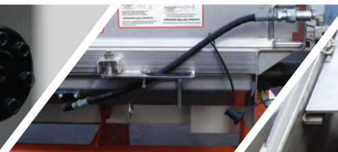
Safety interlock disables auger when opening bottom door or top cover
