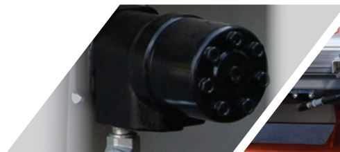
Direct Drive motor drives 6" auger
