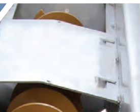
Anti-flow plate prevents material free flow and helps minimize material waste.
