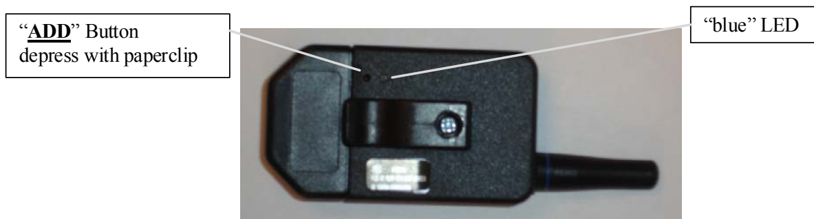
Fig. 2: Transmitter Back Button Assignments
