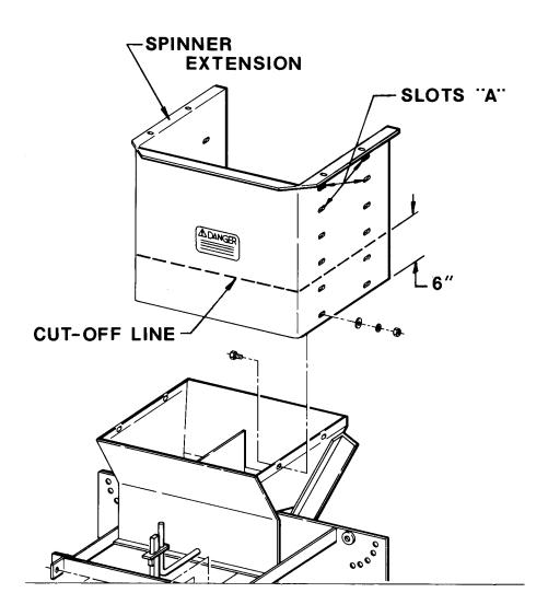
To achieve desired spinner height, assemble by using any of the slots available.
