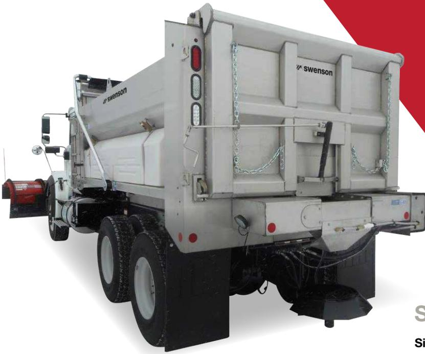
The sloped sides of the APB2S enhance material flow to the conveyor while lowering the center of gravity for improved maneuverability. The cartridge conveyor design helps to protect your equipment while being incredibly easy to service and repair.
