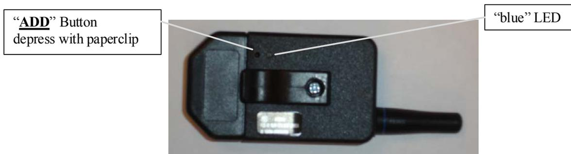
**Fig. 2: Transmitter Back Button Assignments**
