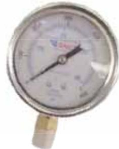
Without a pressure gauge, it is impossible to calibrate your sprayer and keep it calibrated.
